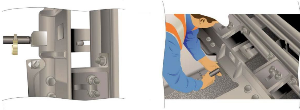
Figure 4: Example of a point clip fitted to the swingnose of VAE points. This type of point uses a special point clip fitted to a plate under the movable swingnose of the points.
