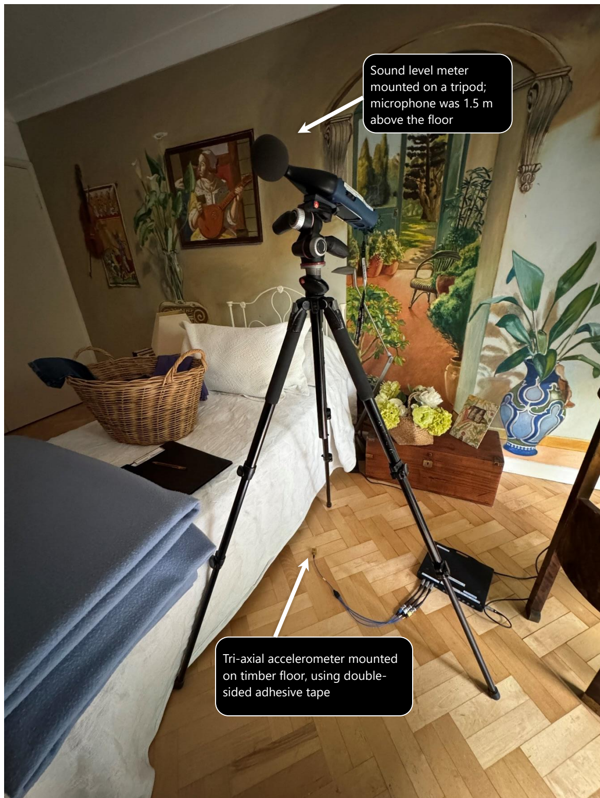
Figure 7-7 Equipment set-up at ■ West Crescent Street, McMahons Point
