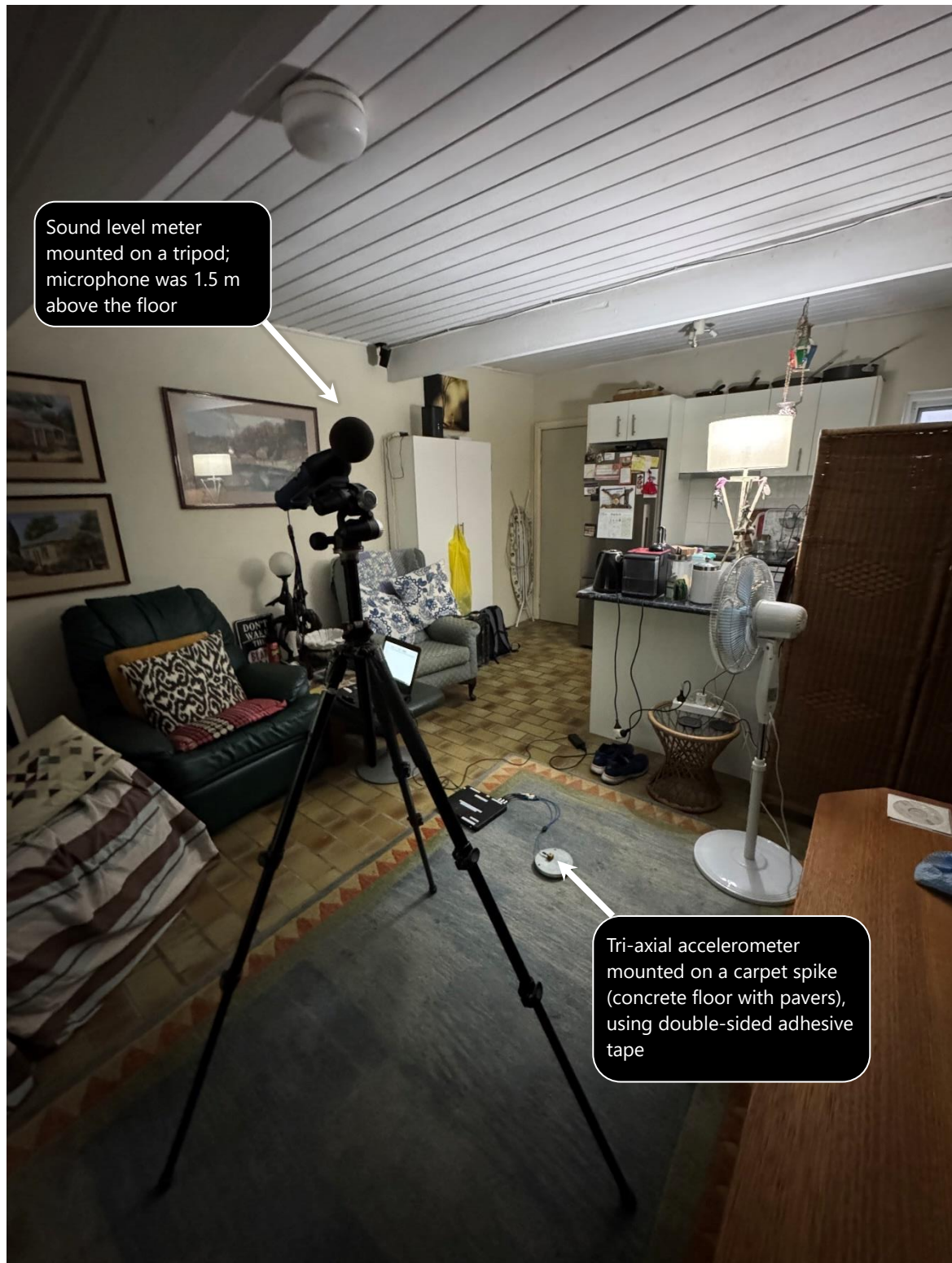
Figure 7-3 Equipment set-up at [REDACTED] Cope Street, Waterloo
