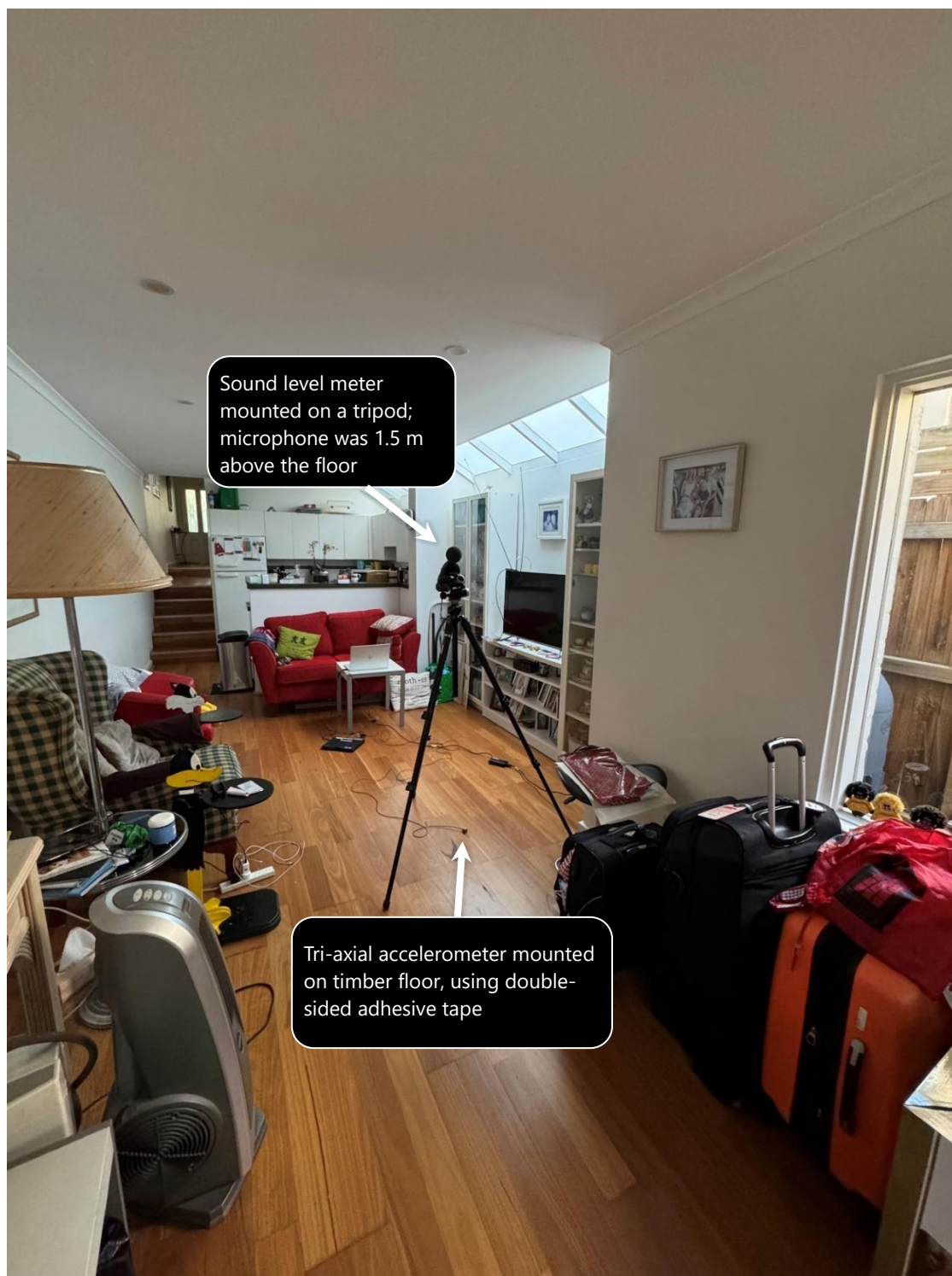
Figure 7-9 Equipment set-up at ■ Hayberry Street, Crows Nest
