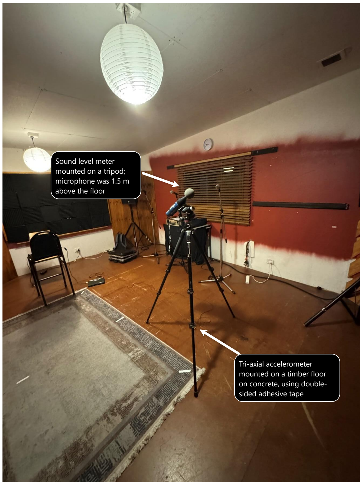
Figure 7-2 Equipment set-up at [REDACTED] Maddox Street, Alexandria (Studio 6)
